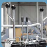
Mech. cross-lever control with rotating function
