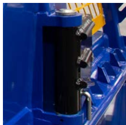
Slewing deflection roller
