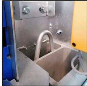
If you want to lift the splitter by the drawbar, use a proper chain hanger or strap. The minimum load capacity must be 300kg higher than the dead weight of the entire log splitter with accessories.
