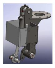
All lubrication spots (marked in RED in the illustration on the left) must be regreased every 8 operating hours.
