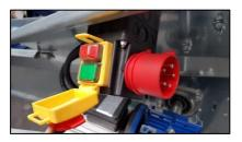
This has 2 buttons, the green button for switching the machine on and the red button for switching it off.
