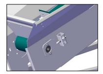
At the bottom, the entire drive roller can be swivelled by means of the threaded rod.
