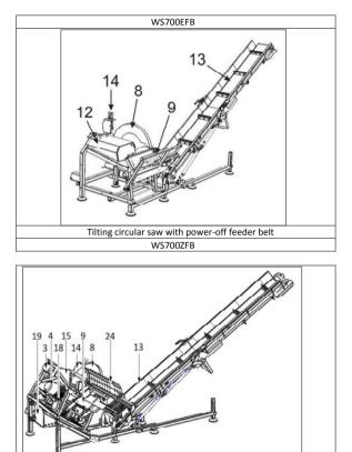
Tilting circular saw with electric feeder belt and independent power
