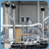
Mech. cross-lever control with rotating function
