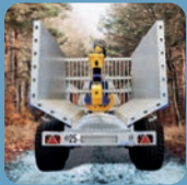
Galvanised brushwood container, formed tube
